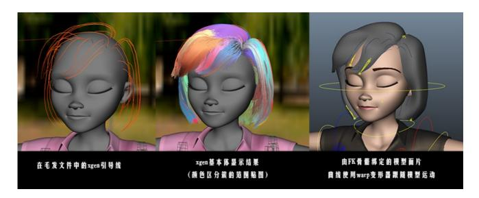
Above we can see that the rig file has a simple mesh for the hair that the animators can see. This is rigged with FK joints for keyframe animation. The hair mesh is then wrap deformed to the curves which we exported from the groom file (III.B.1 above).
