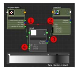
To do the above using a randomized texture map you could output the root\_color through the VRayHairSampler (1), run that through an HSVremap (2) and drive its value attribute with a ramp using shades of grey (3) driven by a "random by strand" attribute (4).
