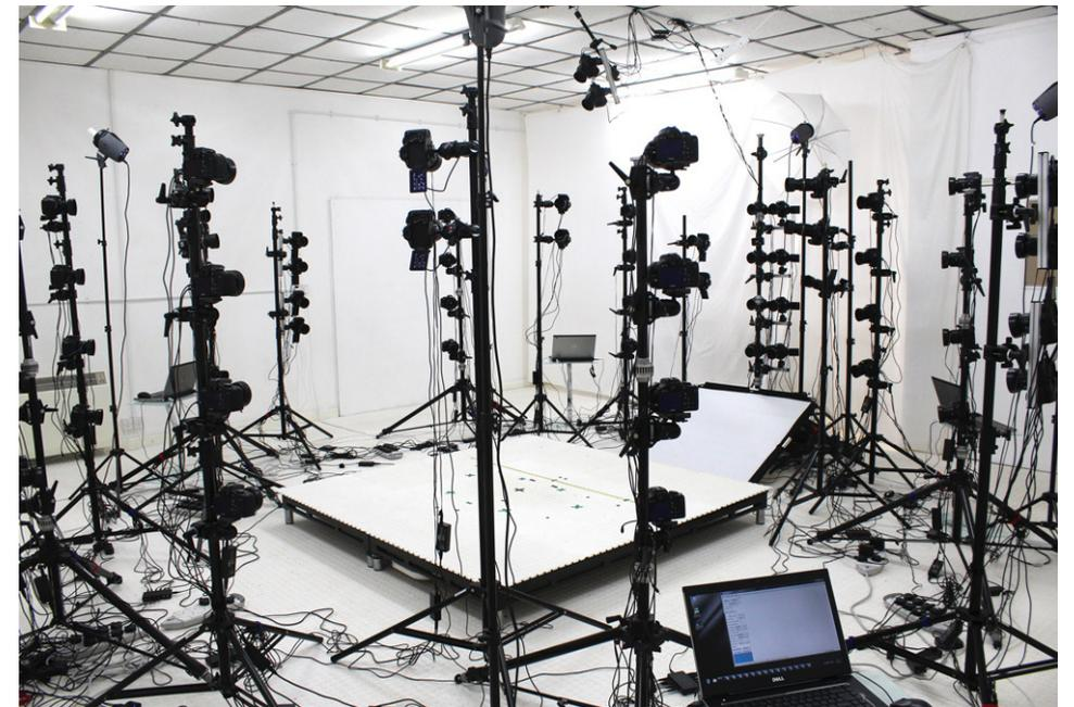
Figure 5: An example of a Photogrammetry Setup containing 72 cameras (Tilbury, 2012).
